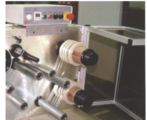
Guarding allows full access to m/c.
